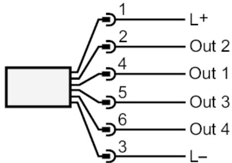
OUT1 : switching output or IO-Link
