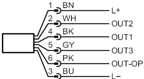
OUT1: IO-Link / switching output
