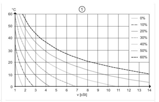
determination of the compensation value Qo for glycol-water mixtures
