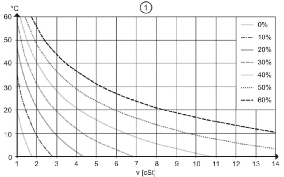
determination of the compensation value  $Q_0$  for glycol-water mixtures
