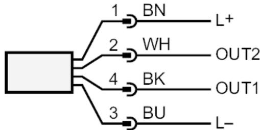
OUT1/IO-Link: Switching output Volumetric flow quantity monitoring
