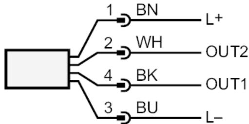
OUT1/IO-Link: Switching output Volumetric flow quantity monitoring
