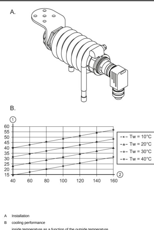
inside temperature as a function of the outside temperature
