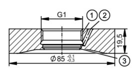
G1 Internal thread Aseptoflex Vario Leakage port sealing area
