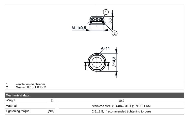
Filter cover including ventilation diaphragm and O-ring
