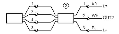
2-wire operation3-wire operationOUT24...20 mA
