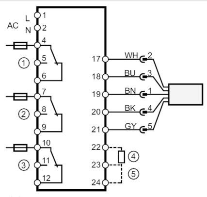
1 = Flow monitoring 2 = Wire monitoring 3 = Temperature monitoring 4 = Power-on delay time
