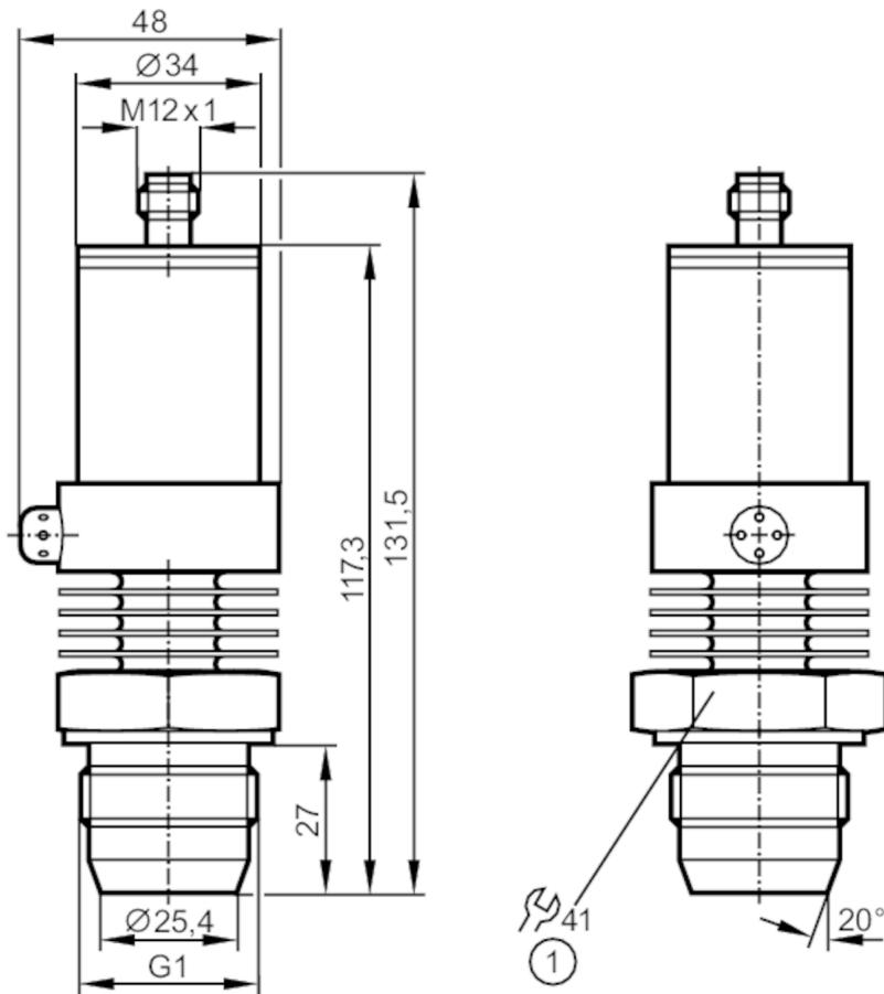
1 Tightening torque 20 Nm
