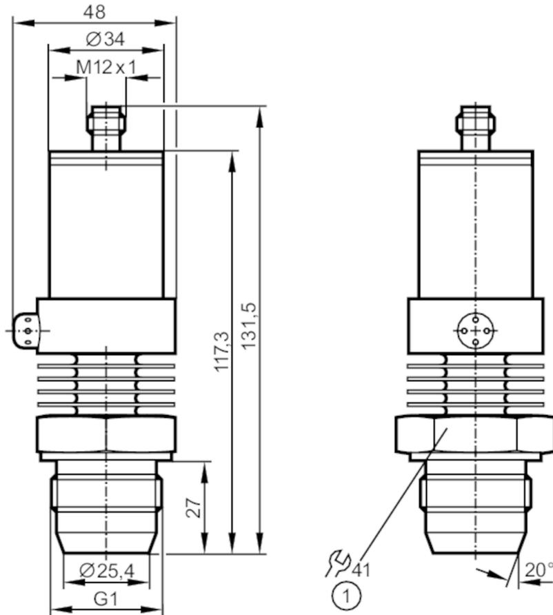
1 Tightening torque 20 Nm
