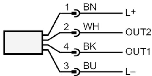
OUT1: switching output IO-Link
