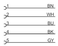
$\begin{array}{ccc} & & & & & & \\ \text{BK} = & & & & \text{black} \\ \text{BN} = & & & \text{brown} \\ \text{BU} = & & & \text{blue} \\ \text{GY} = & & & \text{grey} \\ \text{WH} = & & & \text{white} \\ \end{array}$
