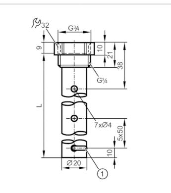
1 fixing bracket for centring piece
