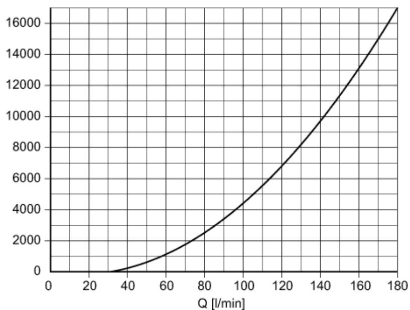
Pressure loss / volumetric flow quantity
