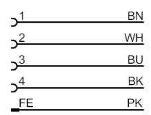
$\begin{array}{ccc} & & & & & & \\ \text{Core colours:} \\ \text{BK =} & & & & \text{black} \\ \text{BN =} & & & \text{brown} \\ \text{BU =} & & & \text{blue} \end{array}$
