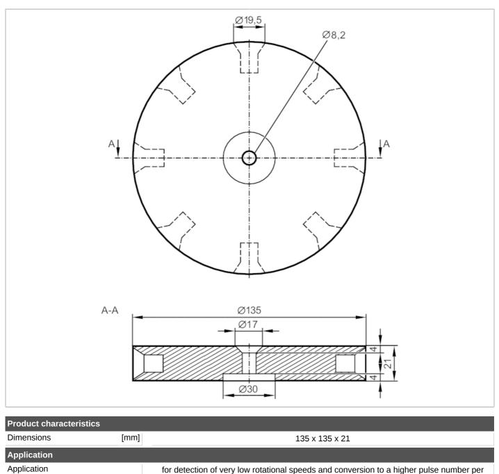
for detection of very low rotational speeds and conversion to a higher pulse number per minute; with even mark-to-space ratio ; e.g. for the use of a frequency-to-current converter
