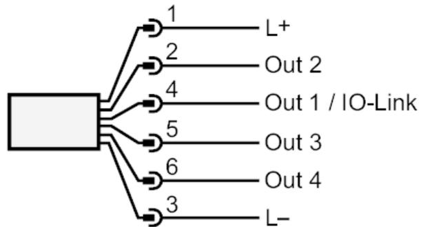
OUT1: switching output IO-Link
