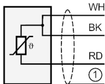
1 = screen not connected to the housing
