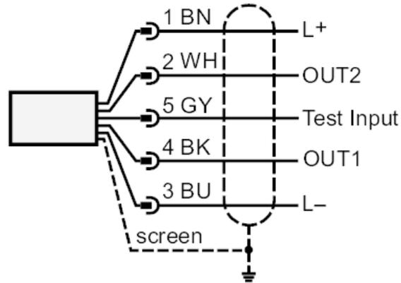
OUT1: switching output / IO-Link
