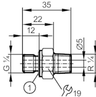
1 Joint d'étanchéité raccord process
