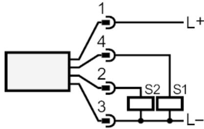
S1: Flow monitoring Temperature monitoring
