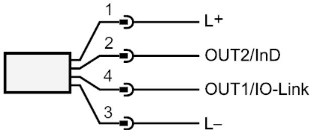
OUT1/IO-Link: switching output volumetric flow quantity monitoring
