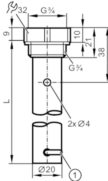
1 fixing bracket for centring piece
