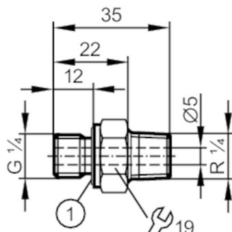
1 Joint d'étanchéité raccord process
