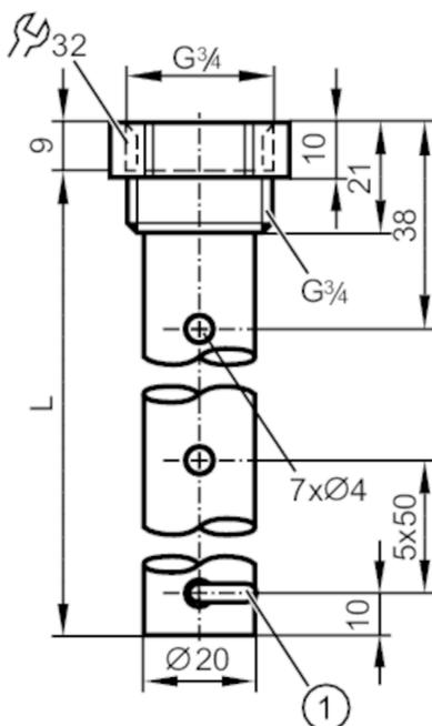
1 fixing bracket for centring piece
