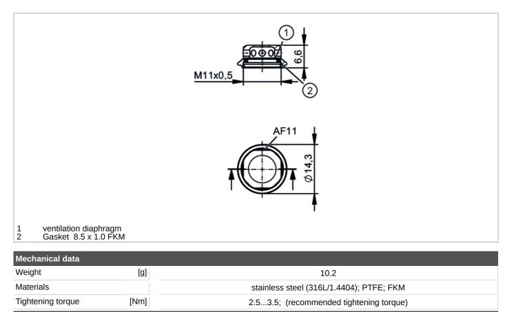
Filter cover including ventilation diaphragm and O-ring
