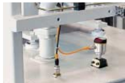
Measurement in the medium: The LK probe is directly immersed in the medium to be monitored.
