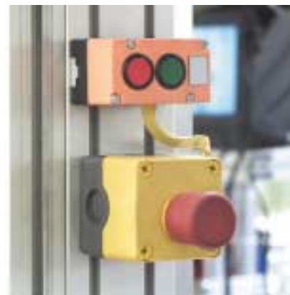
Safety at Work is designed for safety-related applications. Here an E-stop implemented with AS-i.
