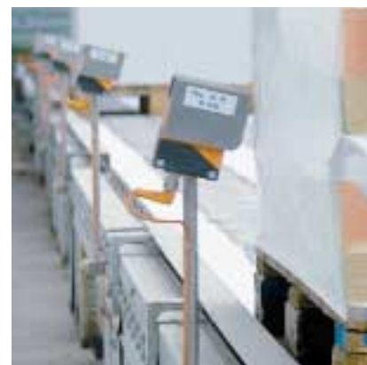
Artificial eyes: Photoelectric sensors are used to detect positions in automation technology.
