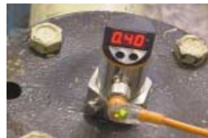
The display: The 7-segment display shows the system pressure at a glance.
