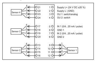
Wiring of the sensors 1...4 (S1...S4) according to the connected unit
