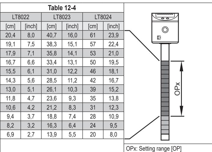
The indicated values for [OP] refer to the distance between OP and the lower edge of the probe.
