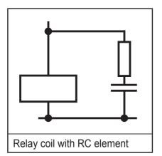
For the dimensioning of the RC element, the following values are recommended:
