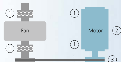
Monitoring of fan and motor, for example with belt transmission
