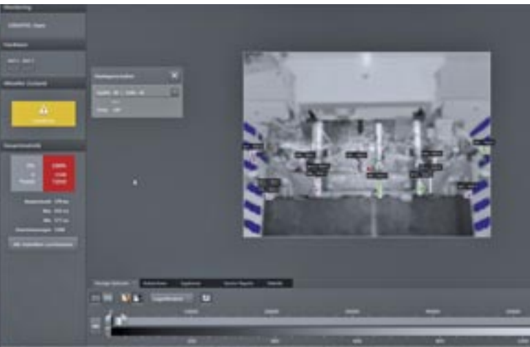
ifm VisionAssistant for parameter setting and visualisation of the O3D camera.
