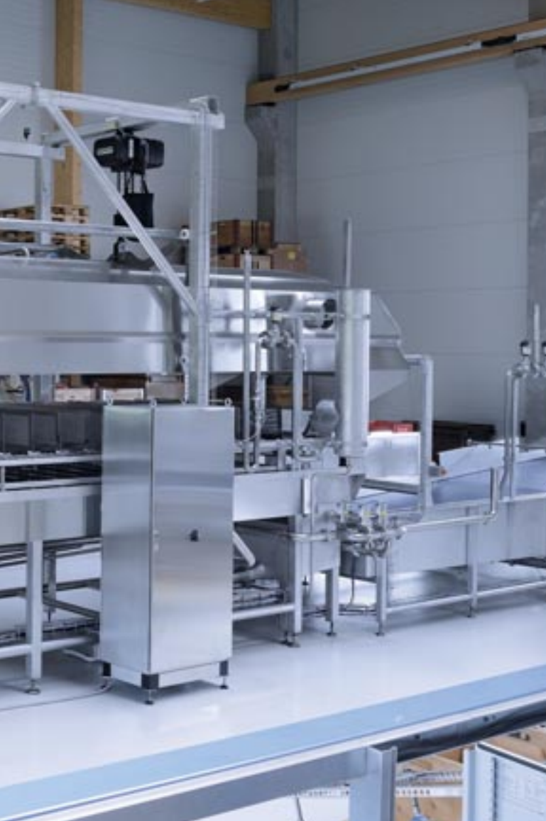
Cooking system type staedler CK1600, manufactured by staedler automation AG. This system will be used to cook spaetzle.
