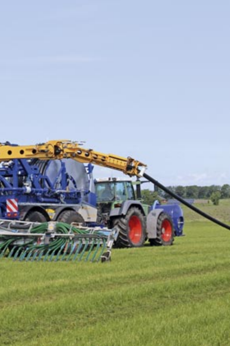
The umbilical injector SRS 1500 is pulled over the field by a tractor to spread slurry.
