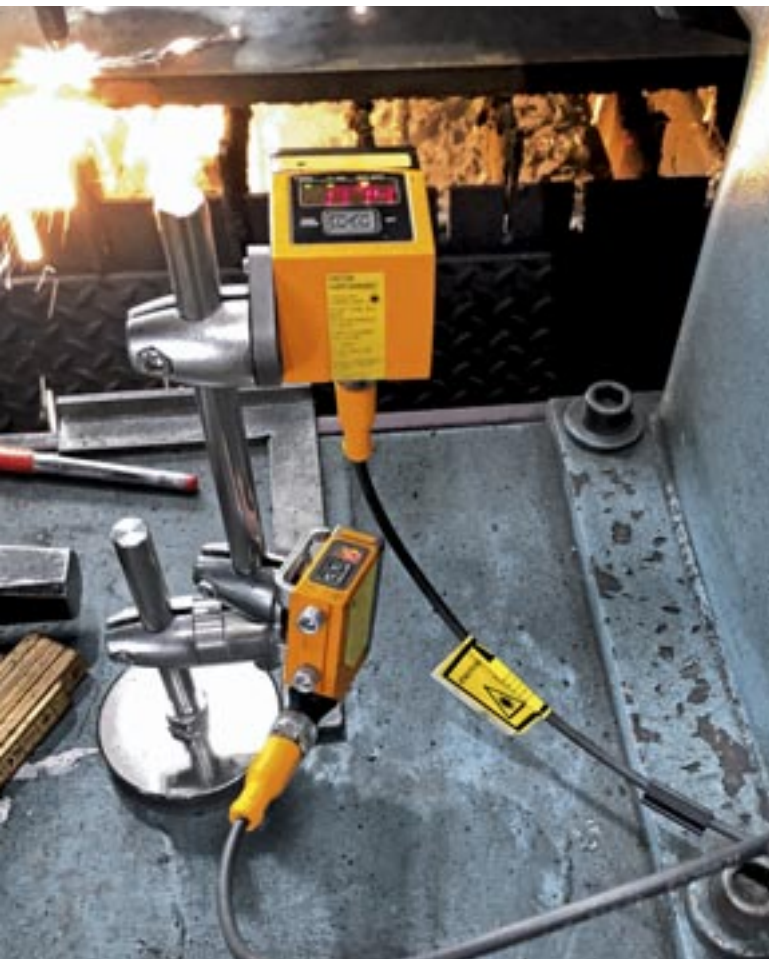
Measure utilisation: ifm sensors detect whether machines are running or in a waiting state.
