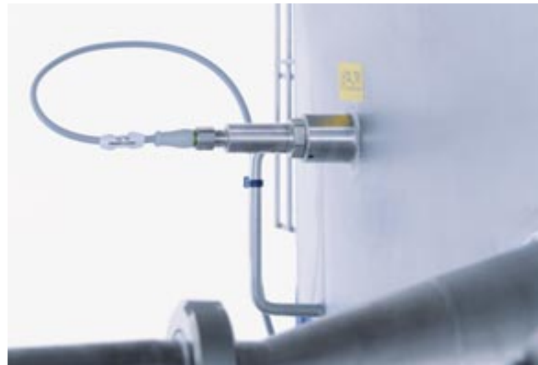
Temperature sensors type TA monitor the required temperature values in the cooker as well as in the cooling bath.
