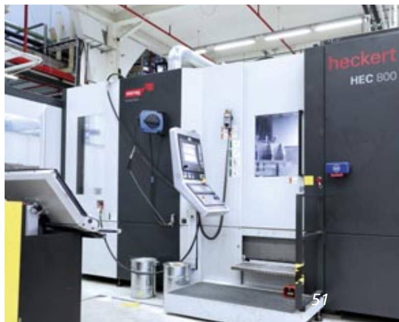
5-axis machine tool to lathe, drill and mill large metal blocks.
