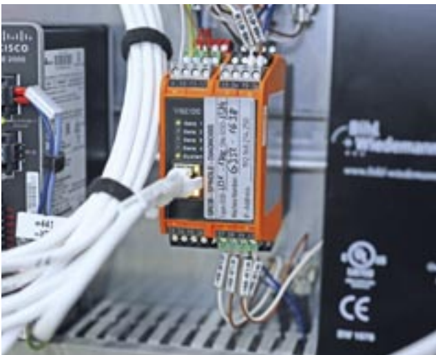
The VSE100 evaluation unit detects the smallest deviations and gives a signal in case of exceeded limit values.
