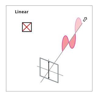
While there are some specific applications where this antenna polarization is beneficial, when investigating an asset tracking program, circular polarization should be used.
