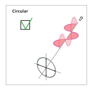
This is significant in discussing the tracking of assets when location, orientation/plane, and distance are never guaranteed. Circular antenna polarization is what allows for tracking portals and UHF mobile automation tracking for intralogistics applications.
