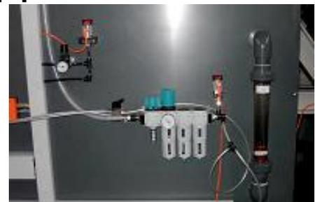
**Figure 20: PN pressure sensors for compressed air measurement**
