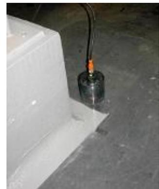
Figure 17: KN series for signalling water penetration
