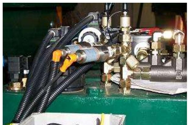
Figure 16: PA9021 pressure transmitter measuring the hydraulic pressure
