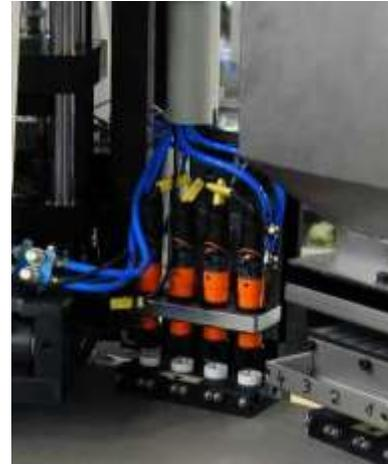
Photo 4: Capacitive proximity switches with probe
