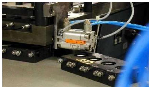
Photo 6: Detection of pneumatic cylinders by means of magnetic cylinder switches
