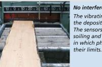
No interference from soiling The vibrating sound transducer reduces the deposit of dust. The sensors operate reliably with heavy soiling and can be used in applications in which photoelectric sensors meet
