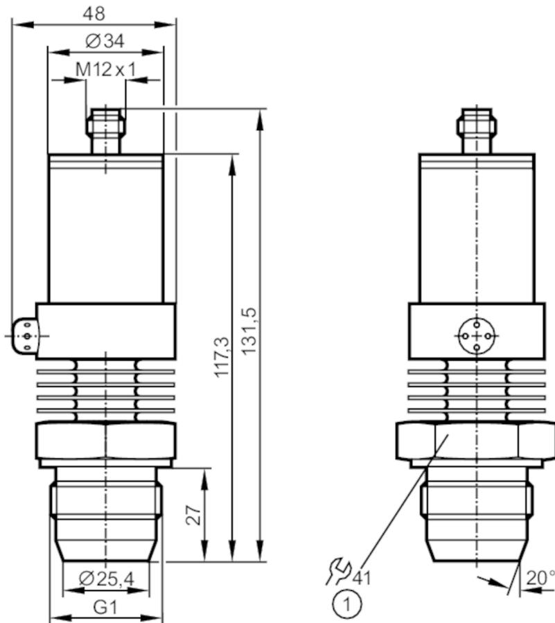
1 Tightening torque 20 Nm
