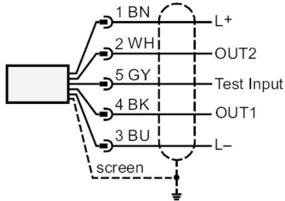
OUT1: switching output / IO-Link
