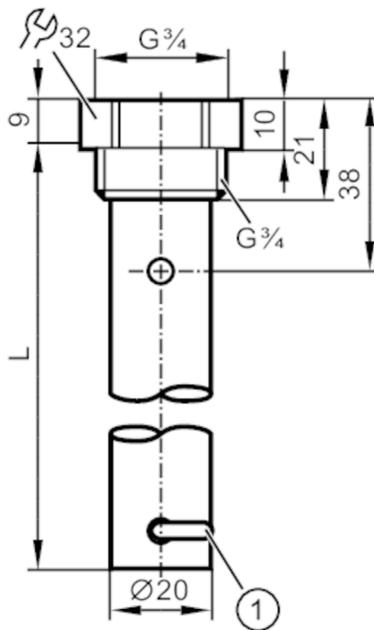
1 fixing bracket for centring piece
