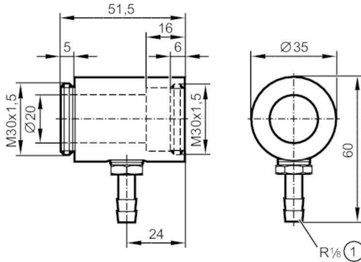
1 Tube nozzle for tube with 8-9 mm bore
