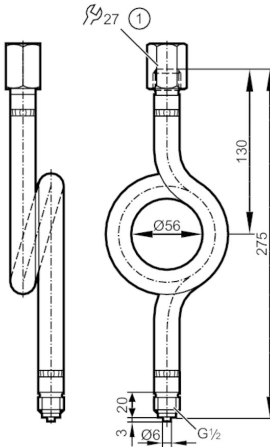
1 clamping sleeve to DIN 16283
