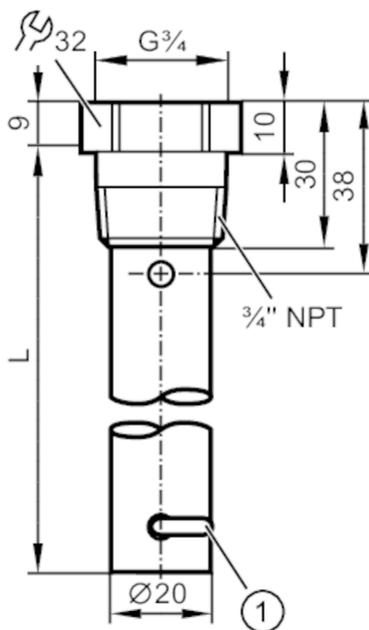
1 fixing bracket for centring piece
