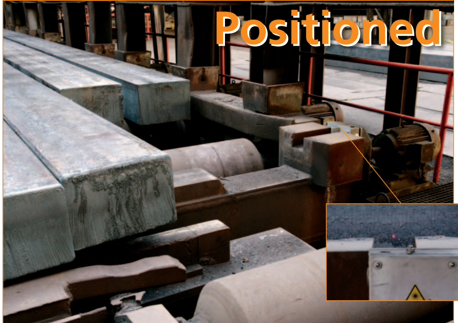
A laser distance sensor efector pmd detects the position of steel blocks.
