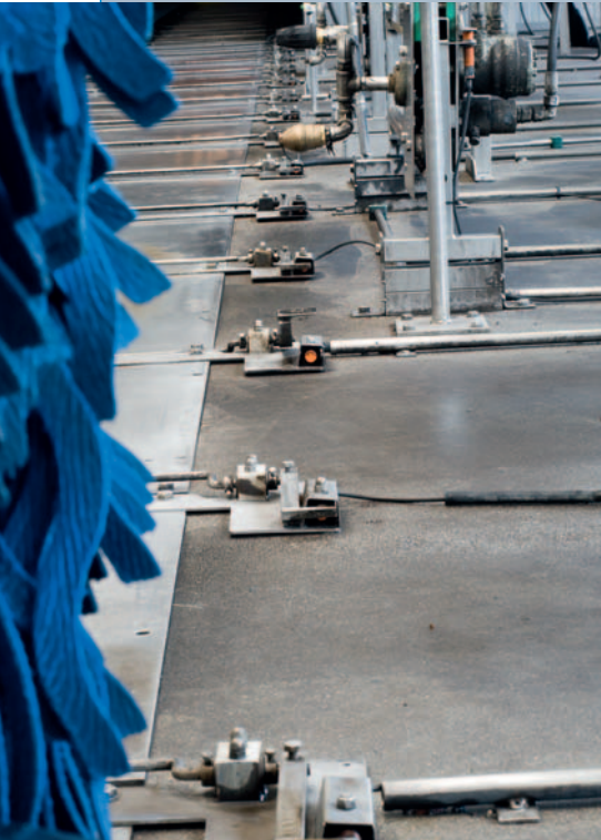
The targets of the release mechanisms, installed at a distance of one metre from each other, are monitored by inductive ifm sensors type IG5564.
