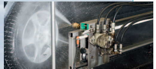
Release mechanisms detect the position of the vehicles at all times and start, for example, the wheel-rim cleaner. The end position of the wheel-rim cleaners is also monitored by ifm sensors
