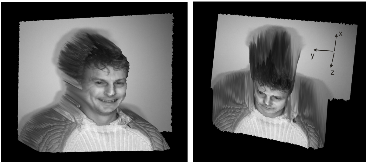
Figure 11: Matching of a high resolution 2D grey scale image with an 3-dimensional depth map.
