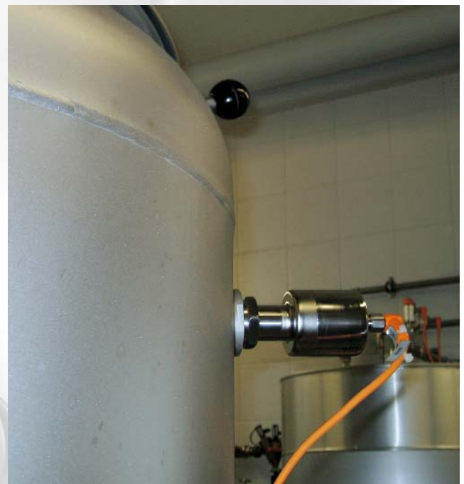
TAD temperature transmitter in hygienic applications for CIP and SIP
